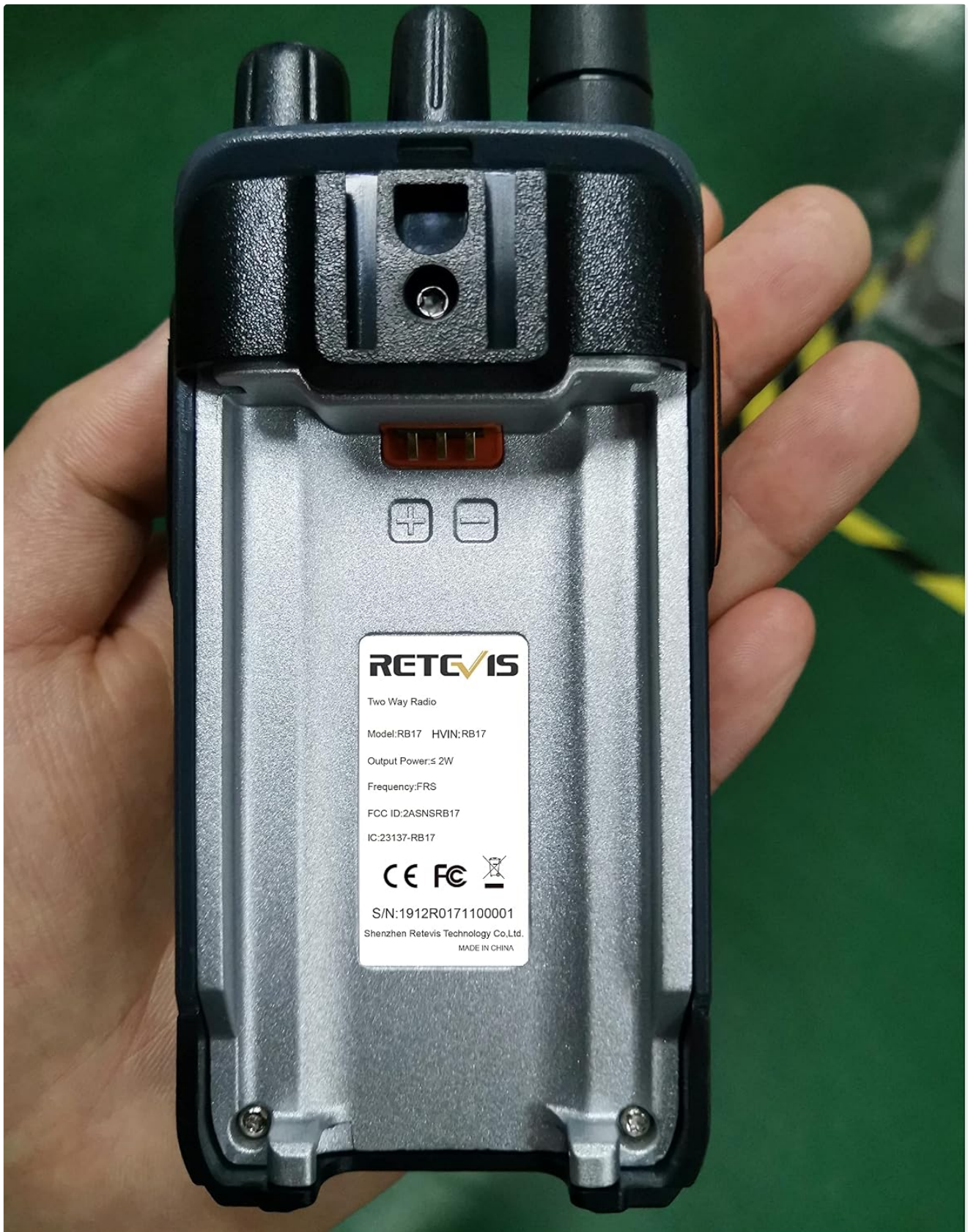
Figure 1: Rear view of the Retevis RB17, displaying model and FCC ID information.
