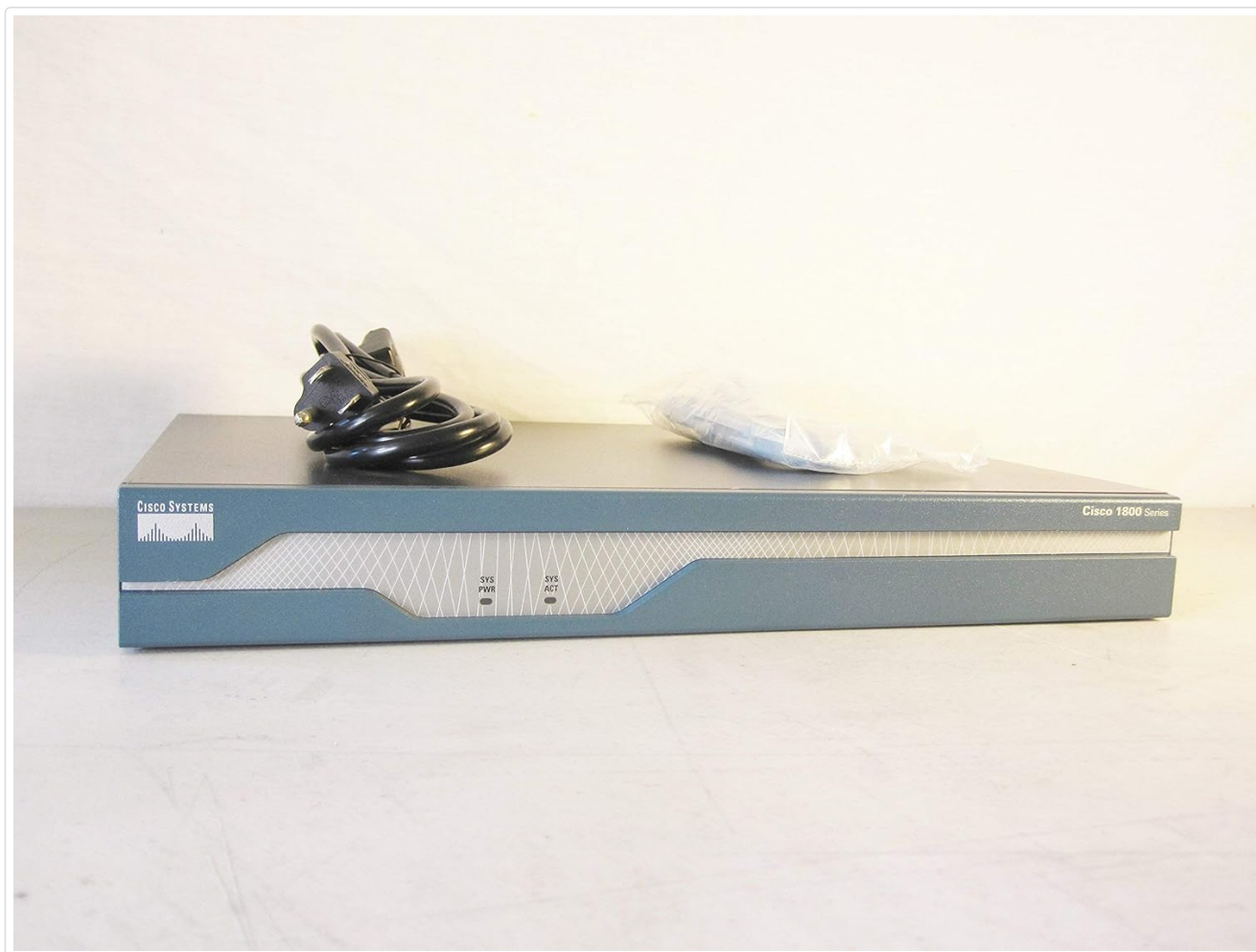
Figure 3.1: Front panel of the Cisco 1841 router with system LEDs.
