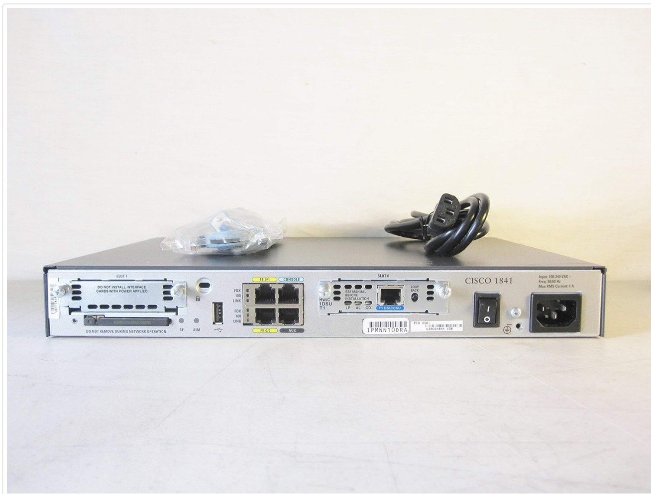
Figure 3.2: Rear panel of the Cisco 1841 router, highlighting Fast Ethernet ports, console port, auxiliary port, WIC slots, and power input.
