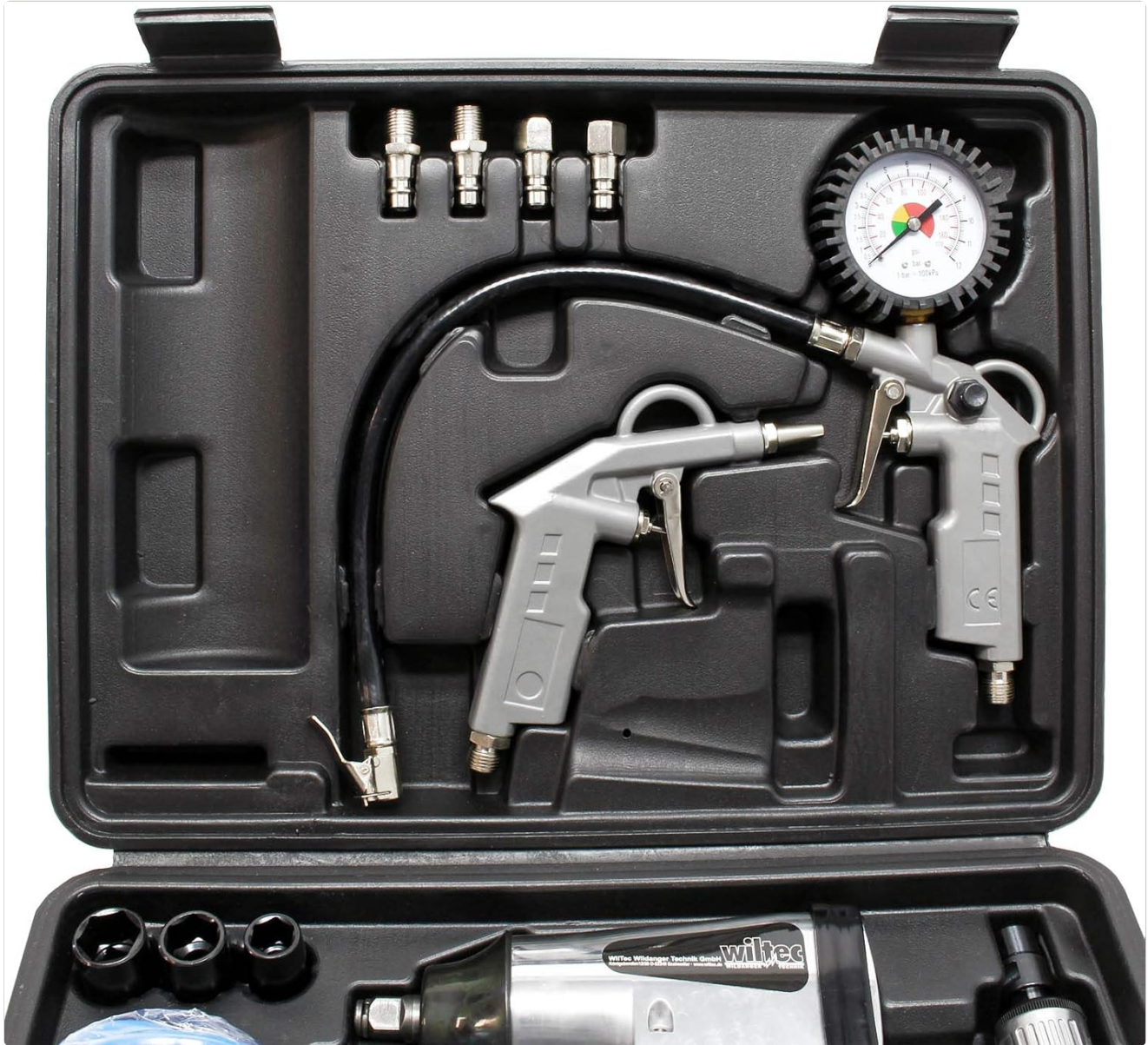
Figure 3: The blow gun and tire inflator with pressure gauge.
