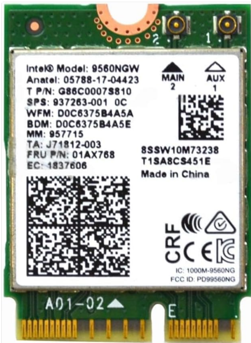
Figure 1: Intel Wireless-AC 9560 M.2 WiFi Card. This image displays the compact M.2 form factor of the card, showing its connectors and labeling.
