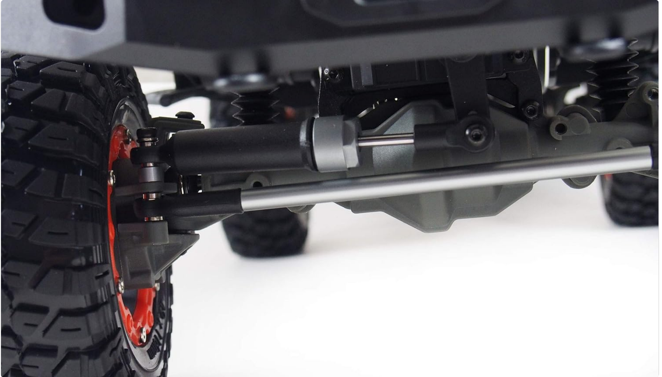
Image: Detail of the damped steering system and front suspension.
