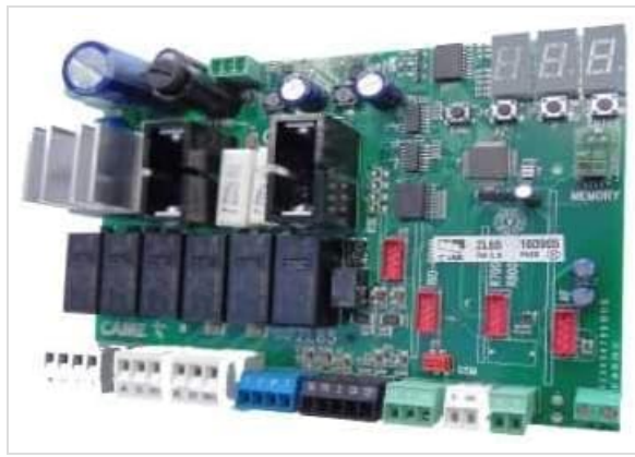
Image 1: The CAME 3199ZL65 electronic control board, showing various components, connectors, and relays.
