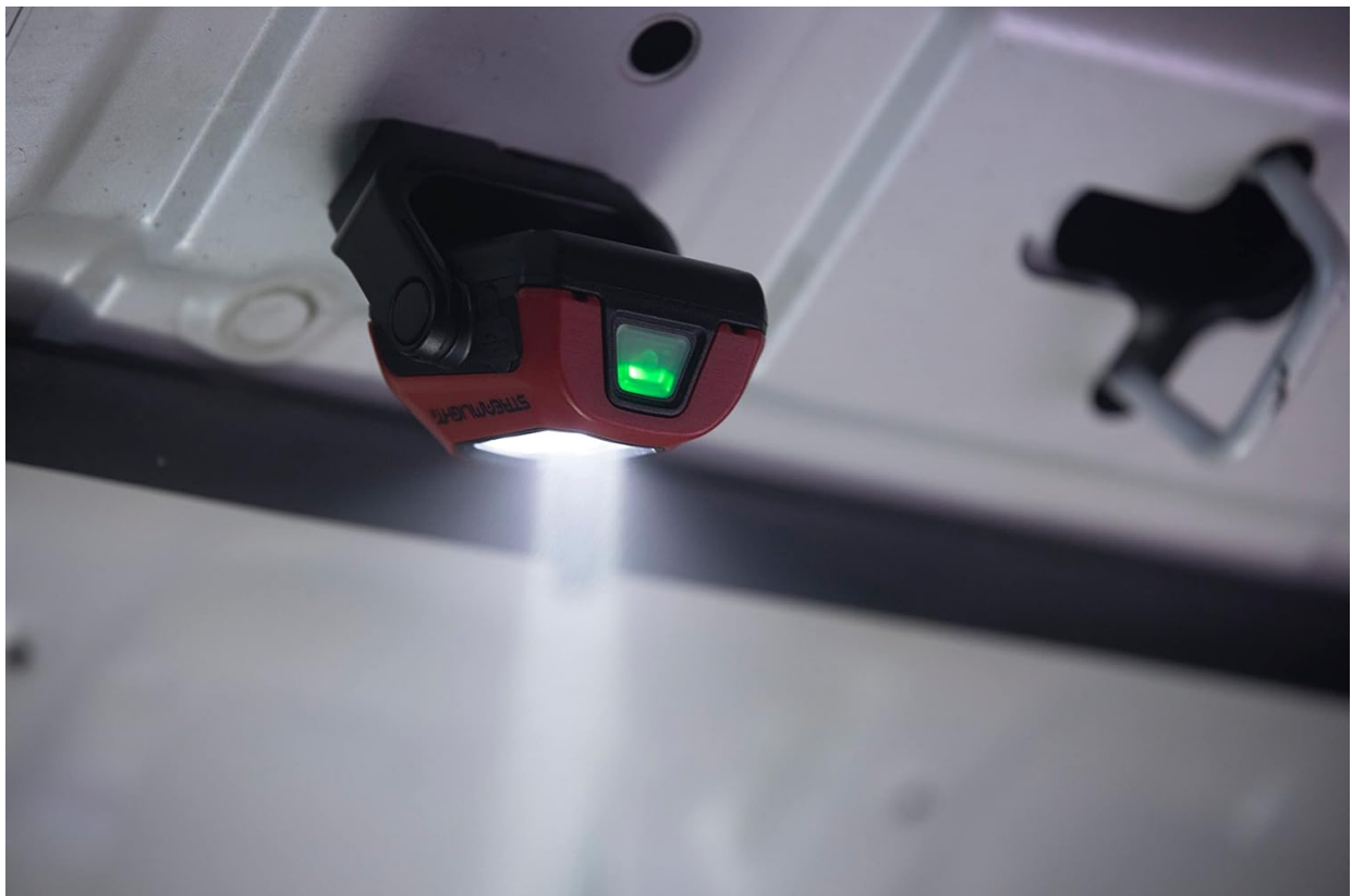
Image: The Streamlight Cyclone in use, magnetically attached to a metal surface to illuminate a work area.
