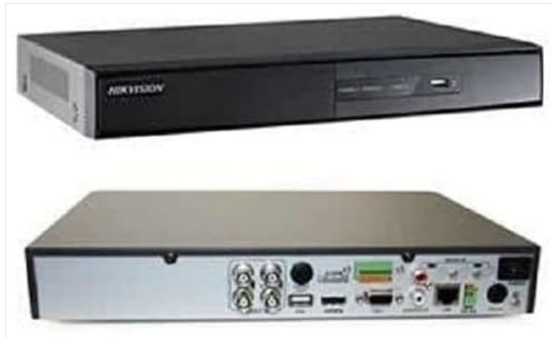
Image 3.1: Front and rear views of the Hikvision DVR, showing various ports.
