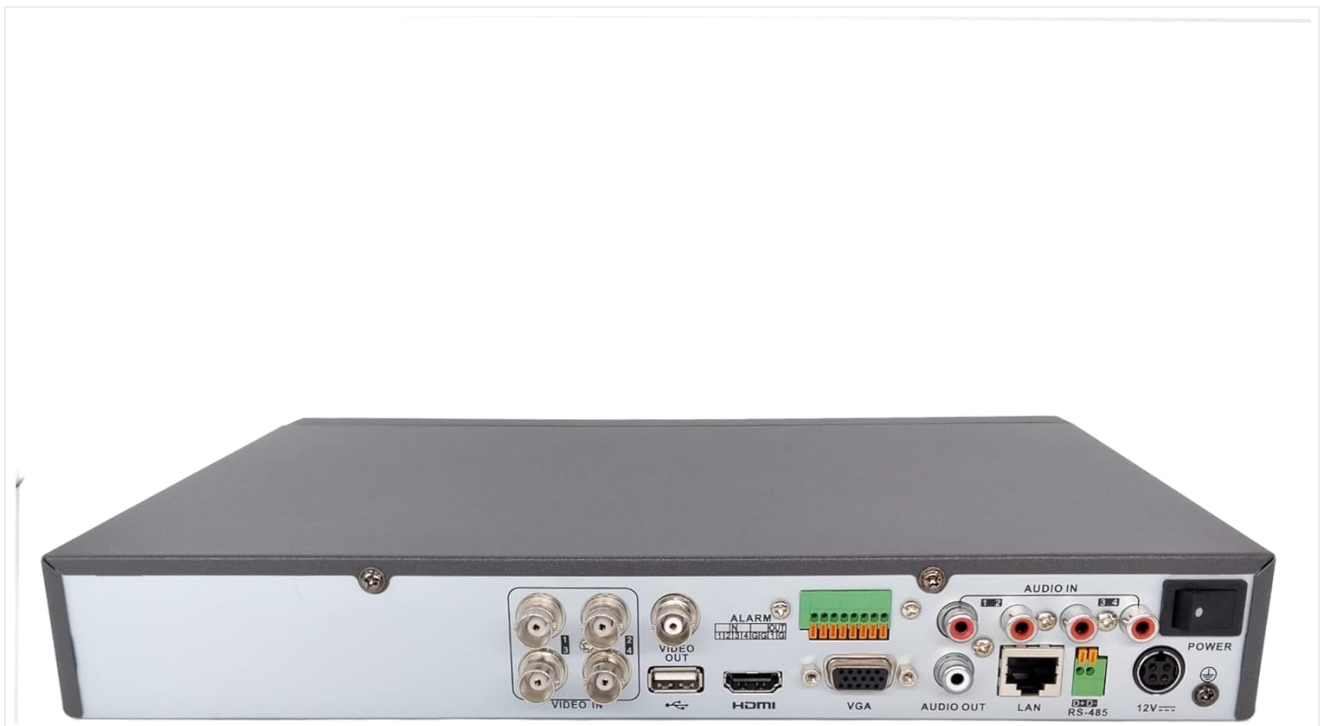
Image 3.2: Detailed view of the DVR's rear panel connections.
