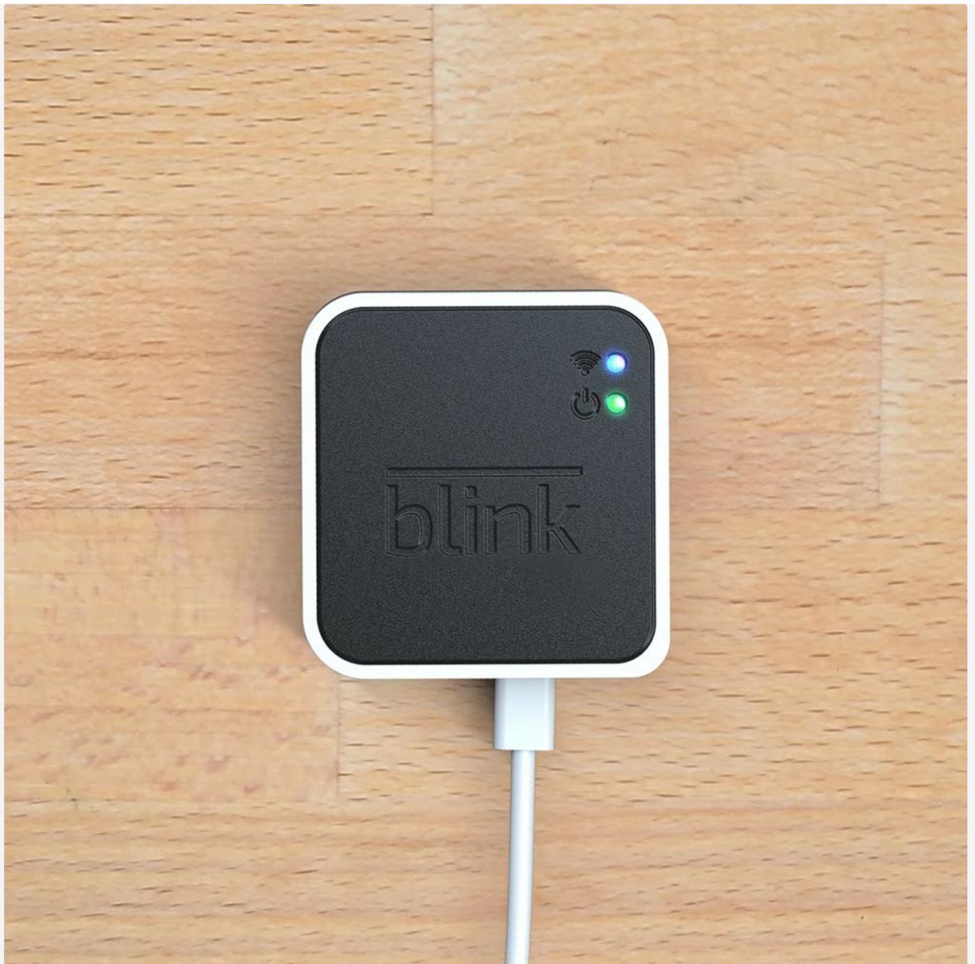
Figure 2.1: The Sync Module 2 connected to its power cable. Ensure a stable power source for continuous operation.
