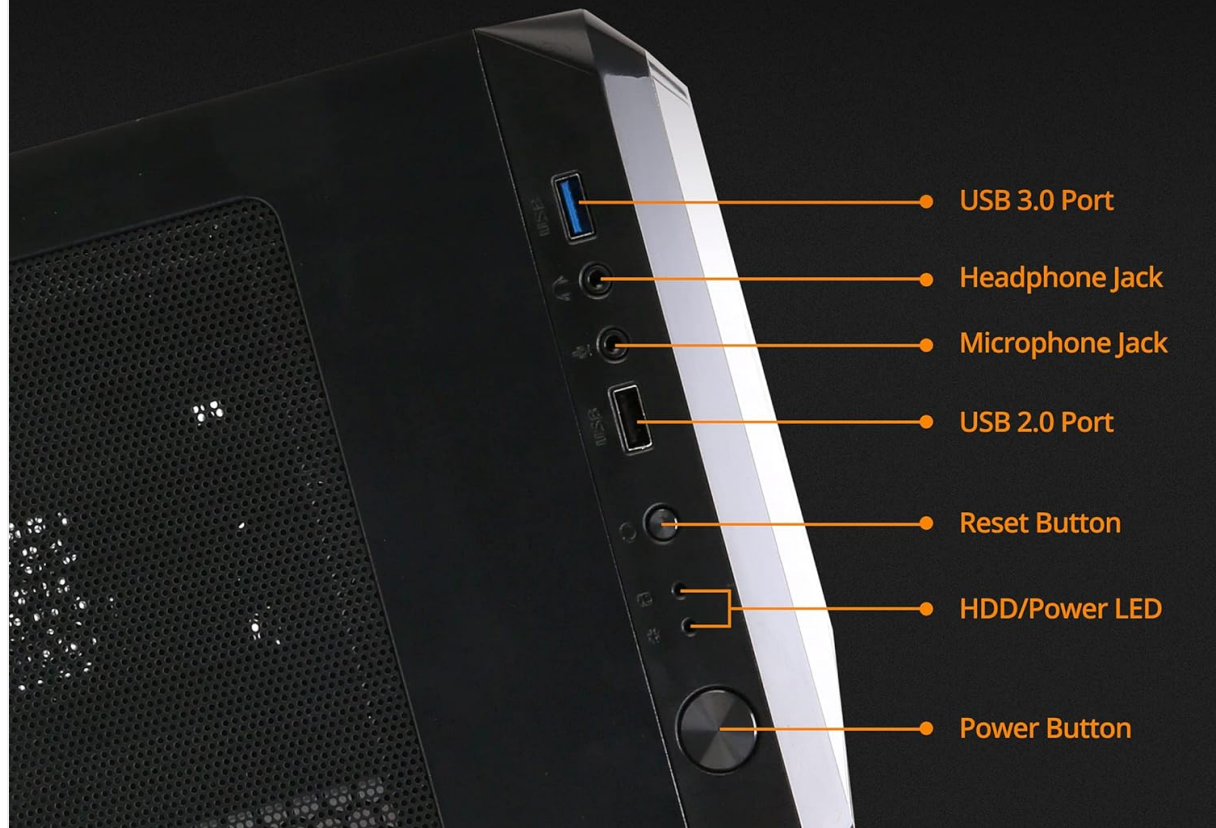
Figure 4.1: Front I/O Ports. This image displays a close-up of the top-front panel of the Zalman S4 PC case, highlighting the various input/output ports and buttons. From left to right, these include a USB 3.0 Port, Headphone Jack, Microphone Jack, two USB 2.0 Ports, a Reset Button, HDD/Power LED indicators, and the Power Button.
