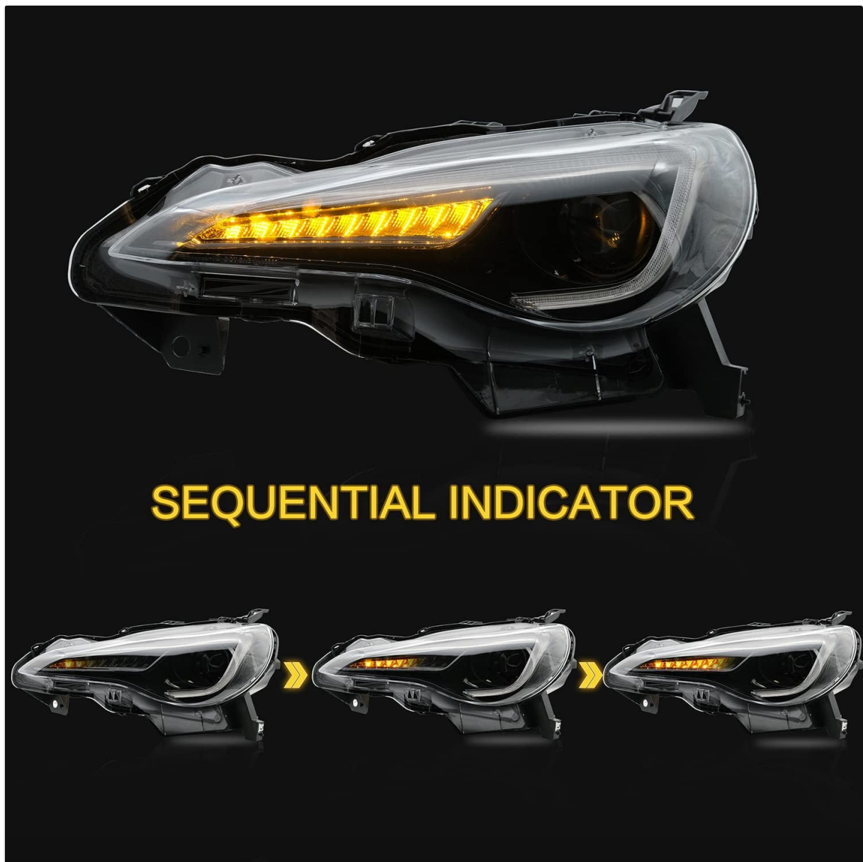
Image 5.1: Illustration of the sequential illumination pattern of the turn signal indicator.
