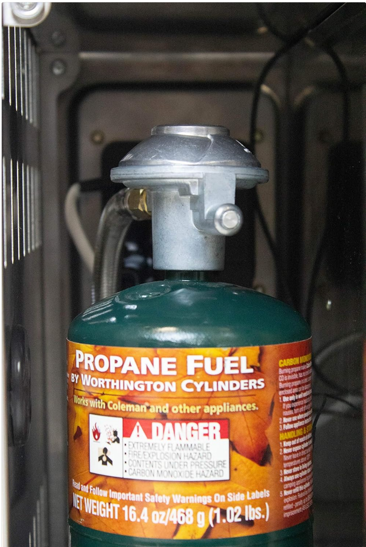
Image: A propane fuel cylinder connected to the grill's gas regulator, illustrating the fuel connection point.
