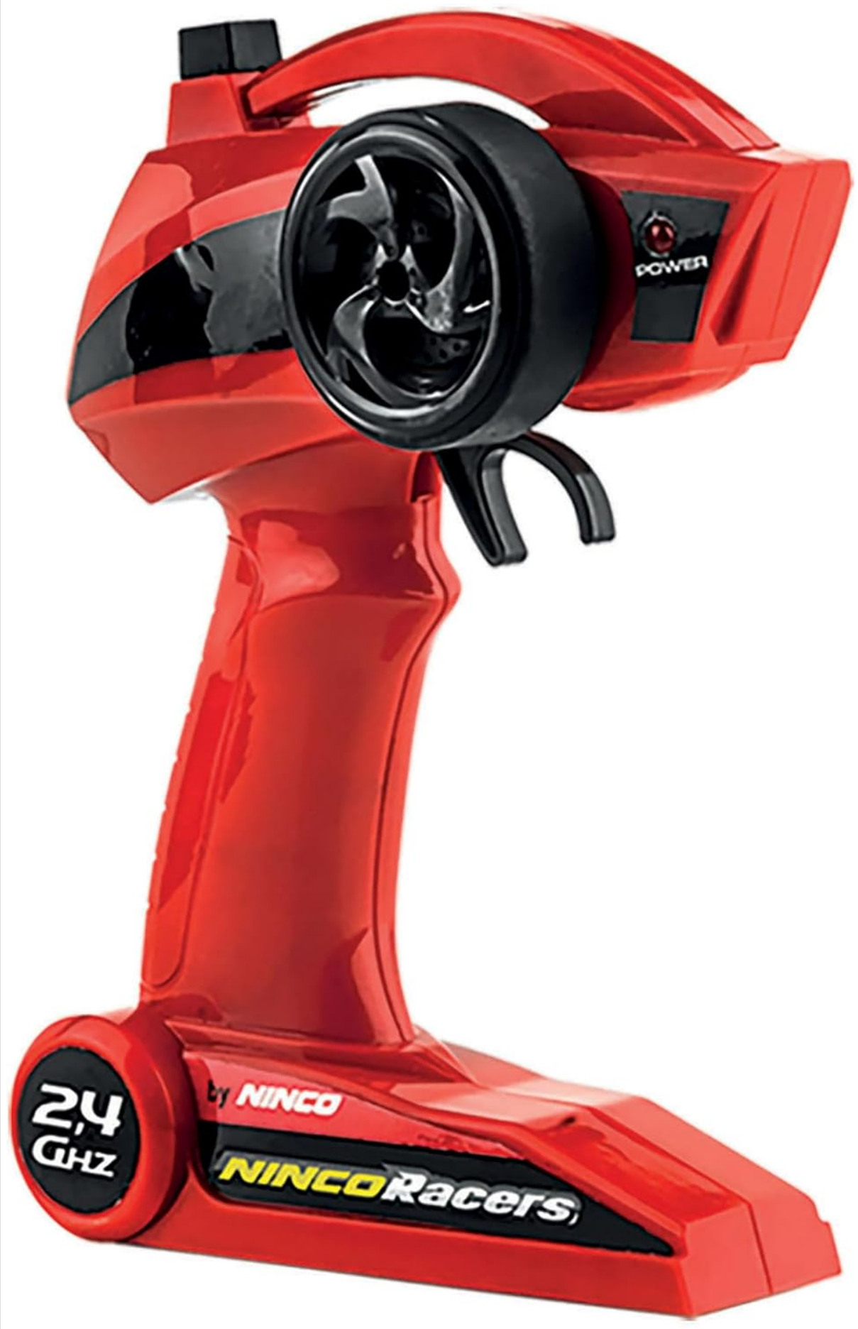
Figure 2: The 2.4 GHz remote control transmitter for the Ninco NincoRacers car.
