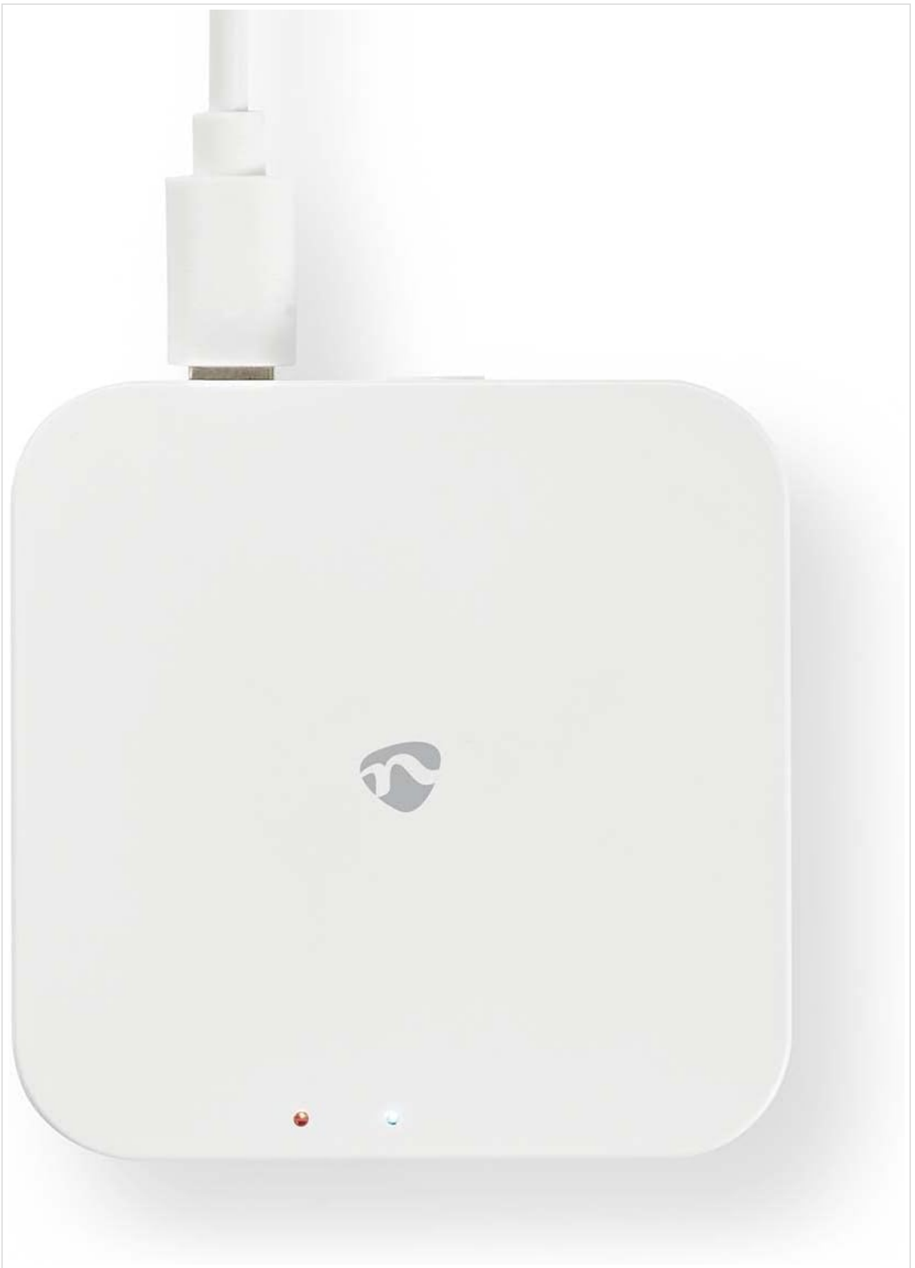
Image 5.2: Top view of the gateway, showing the status indicator lights.
