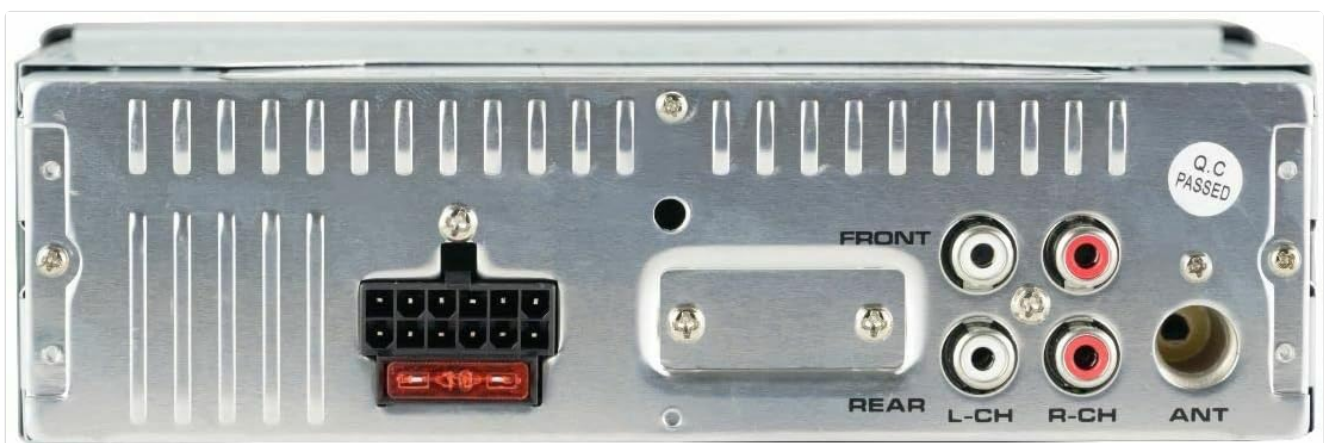
Figure 3.3: Rear view of the receiver with wiring harness port, RCA outputs, and antenna input.
