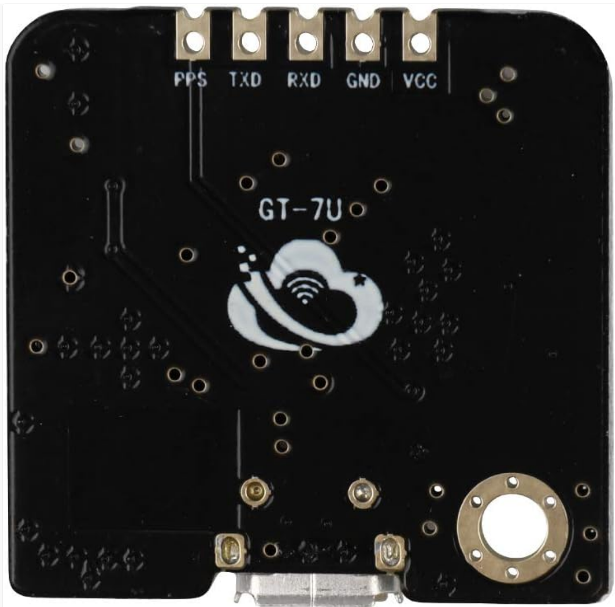
Image 4.2: Pinout labels on the GT-U7 module: PPS, TXD, RXD, GND, VCC.
