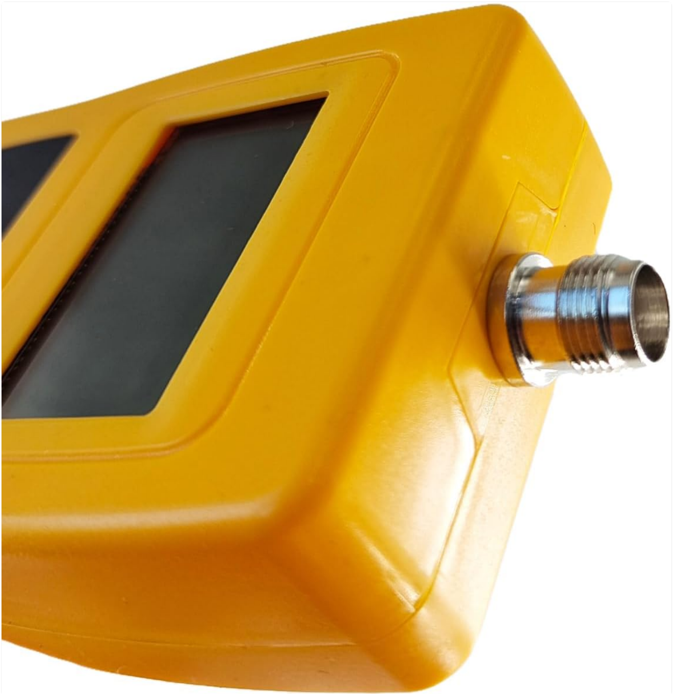
Image 4: A close-up view of the probe detached from the main unit, showing the connector port.
