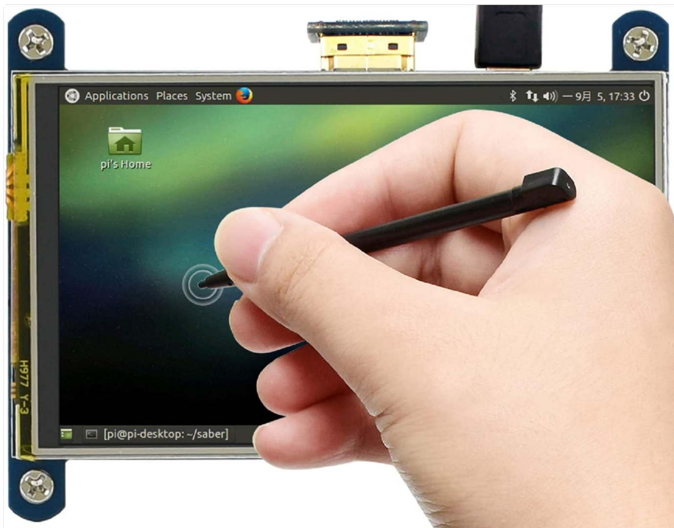
Figure 4: Using the resistive touch screen with a touch pen.
