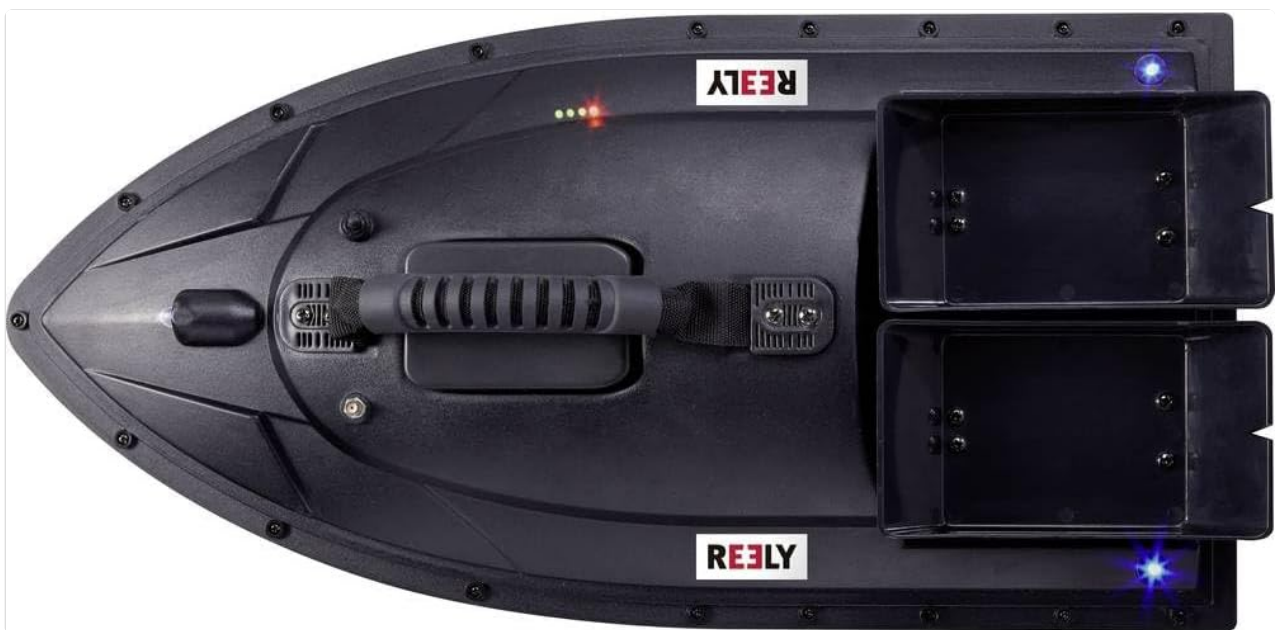
Image: Top view of the bait boat showing the two bait hoppers.
