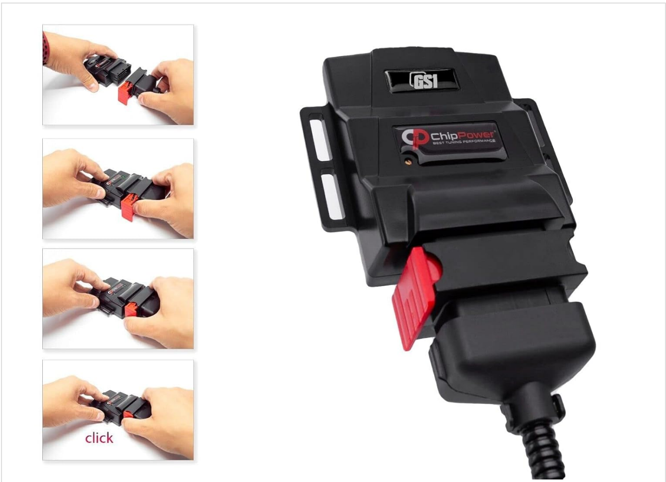
Image 4.2: A visual guide demonstrating the secure connection process of the module to the cable, ensuring a firm 'click'.
