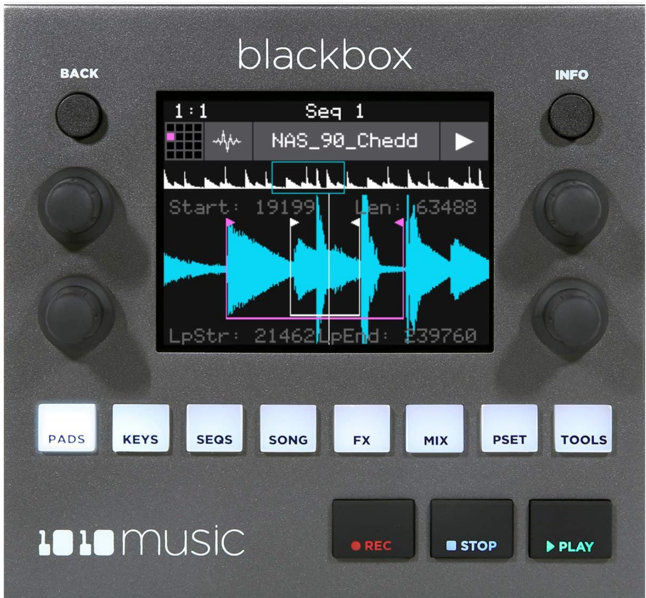
Figure 3: Front view of the Blackbox, showing the touchscreen display, control knobs, and function buttons.
