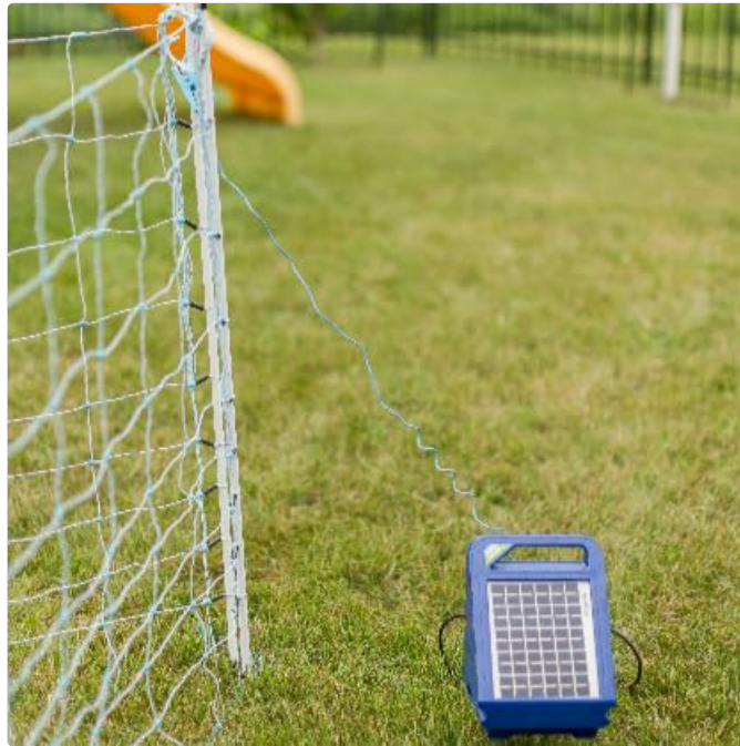
Figure 3: The energizer connected to the electric fence netting and a ground stake.
