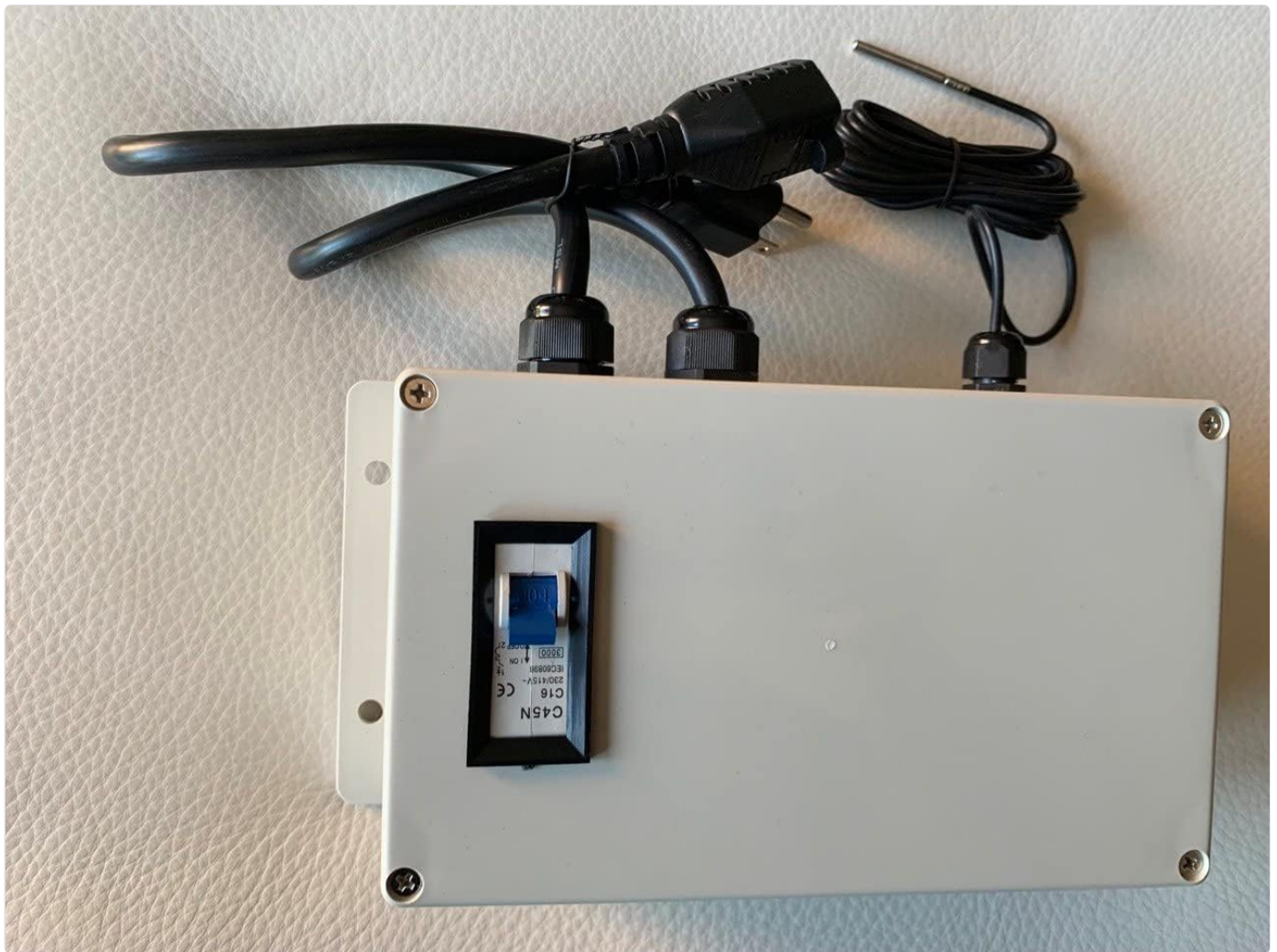
Figure 4: Top view illustrating the power input, appliance output, and sensor connections.
