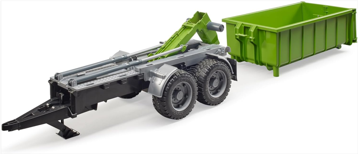
Figure 4: The trailer chassis with the container trough detached.
