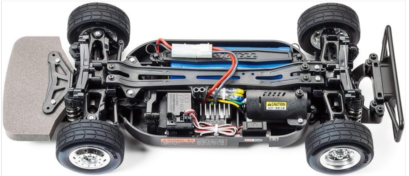
Figure 3.3: Underside view of the Tamiya TT-01E chassis. This image displays the layout of the drivetrain, suspension components, motor, electronic speed controller (ESC), and battery compartment, illustrating the robust design.
