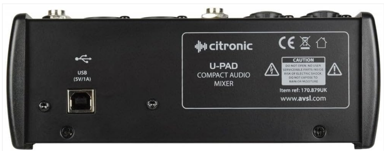
Figure 3: Rear view of the mixer, highlighting the USB (5V/1A) input port and important caution labels regarding servicing and moisture exposure.
