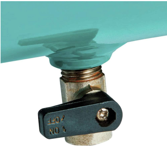
Figure 3.4: Drain Valve of Makita MAC100Q Air Compressor. A close-up view of the tank's drain valve, crucial for releasing condensed moisture and maintaining the tank's integrity.
