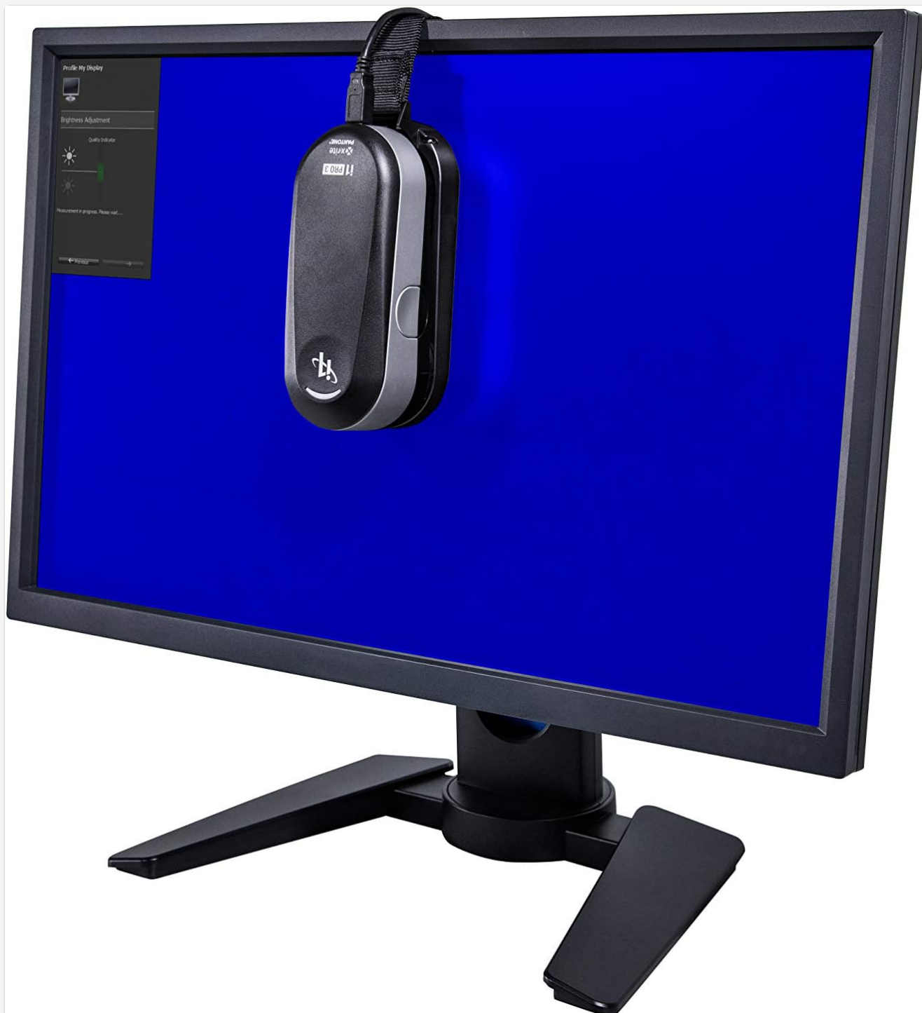
Figure 4.1: The i1Basic Pro 3 spectrophotometer positioned on a monitor screen, ready for display calibration.
