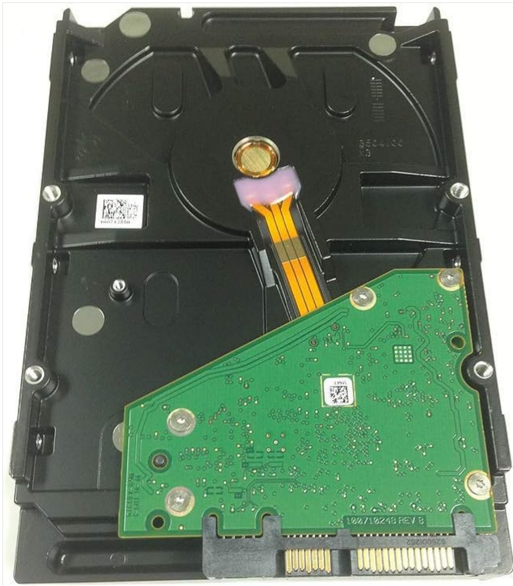
Figure 2: Bottom view of the hard drive, illustrating the SATA data and power connector ports.
