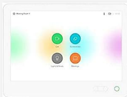
Figure 1: Front view of the Cisco Touch 10 Control Unit displaying its main interface with icons for Call, Share, Lights & Shades, and Messages.
