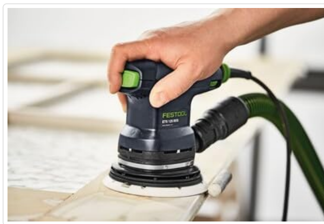
Figure 5: Proper technique for operating the sander on a workpiece.
