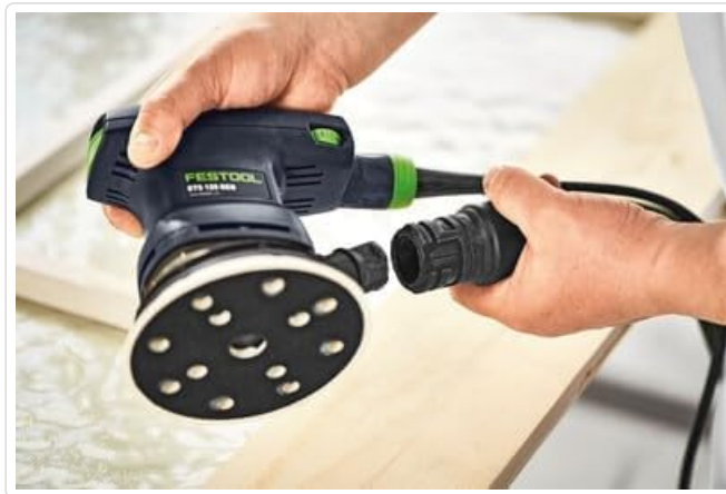
Figure 3: Connecting a dust extraction hose to the sander.
