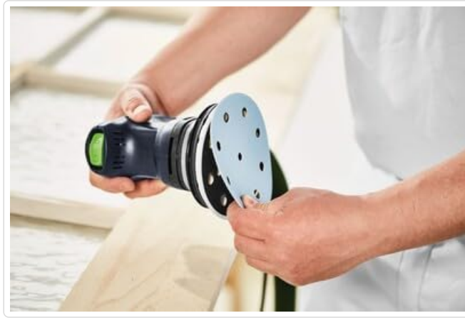
Figure 2: Attaching a sanding disc to the sander's StickFix pad.
