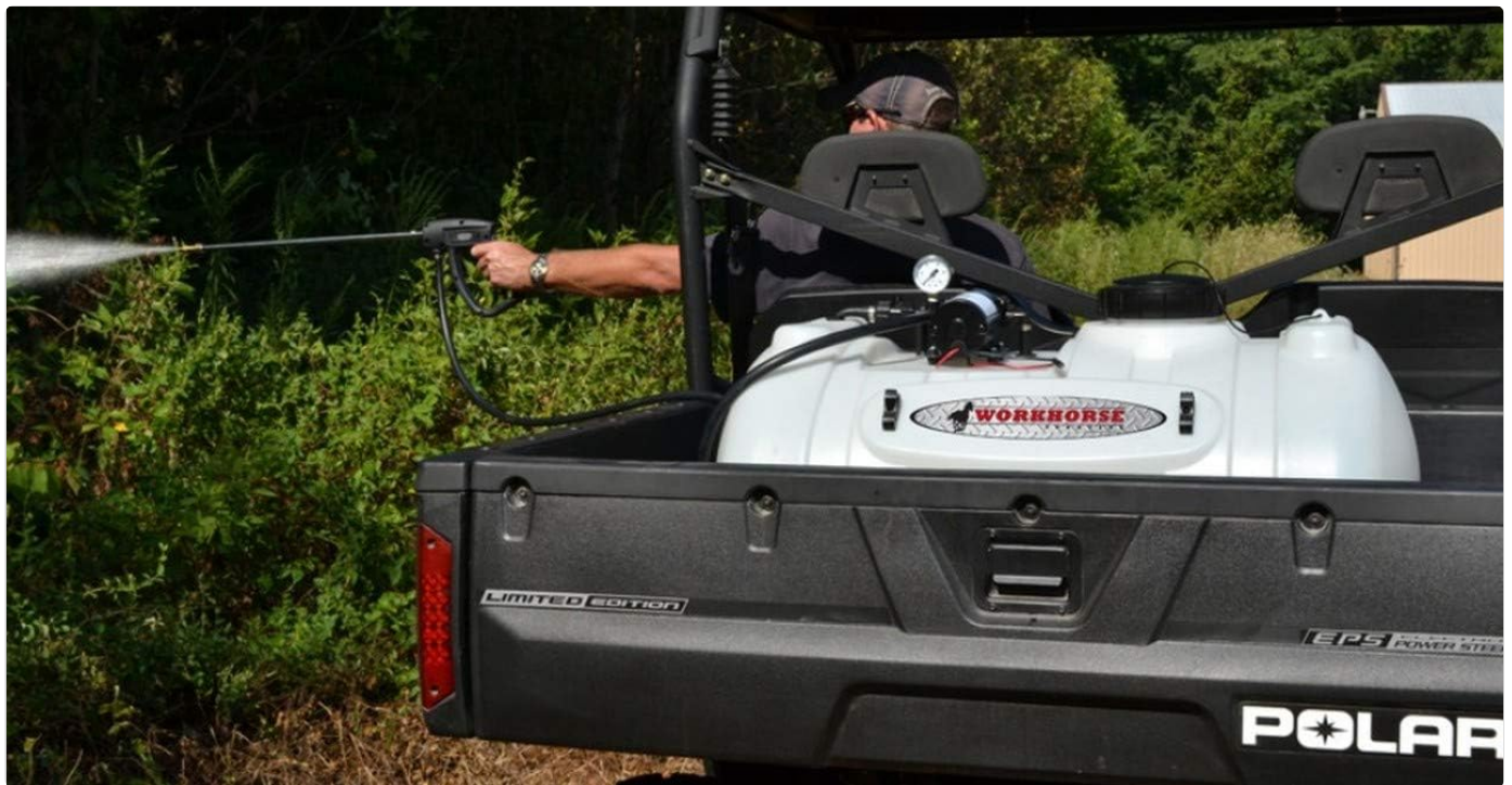
Figure 2: The Workhorse 40 Gallon Deluxe Spot Sprayer mounted in the bed of a utility vehicle during operation.
