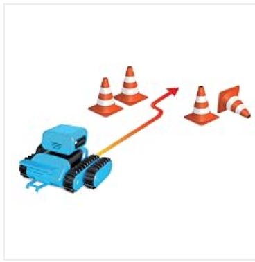
Image: The OWI RE/CO Robot demonstrating its patrol mode, autonomously moving along a path indicated by an arrow, avoiding orange traffic cones using its infrared sensor.
