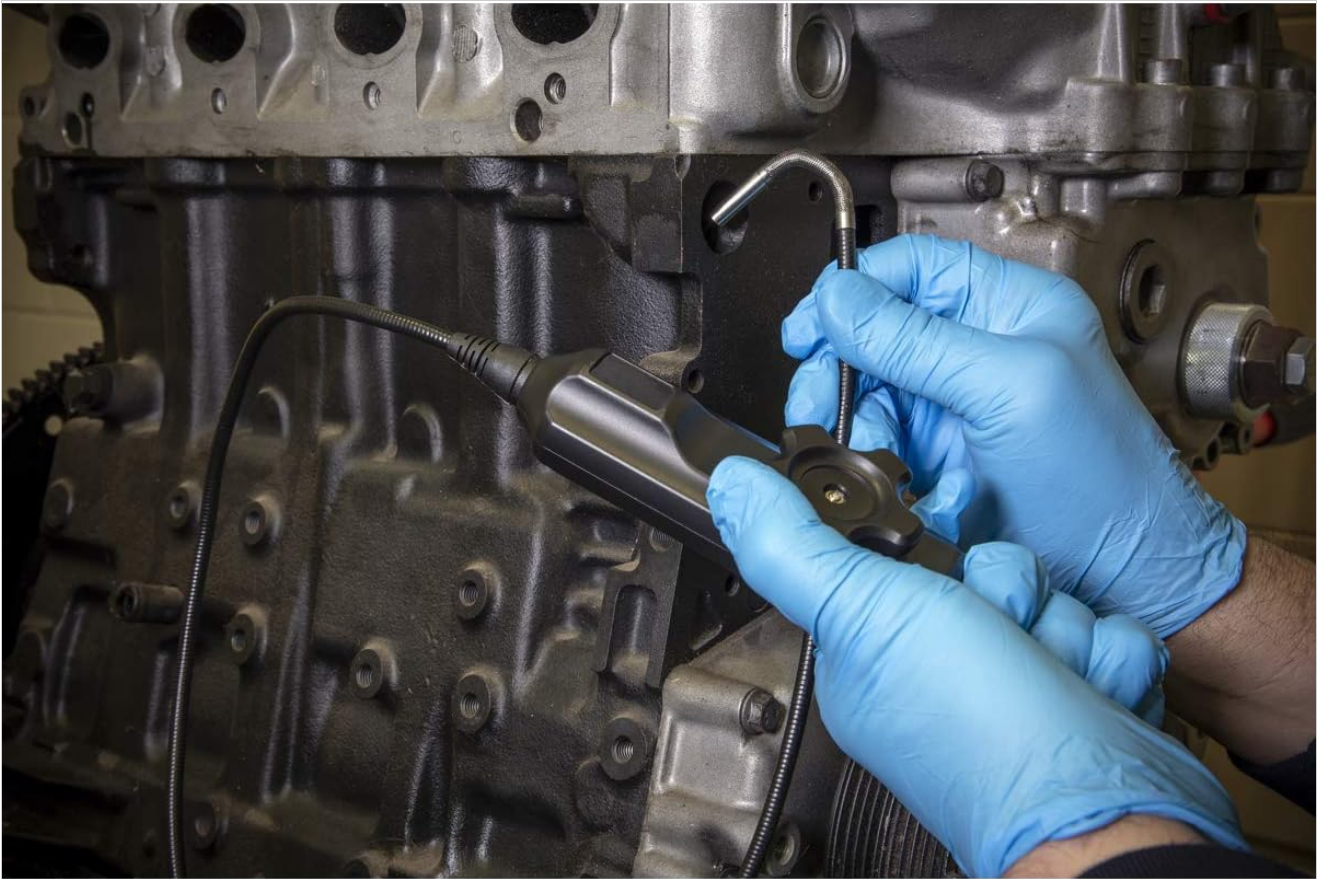
Image: A user wearing blue gloves operates the Sealey VS8233A borescope, guiding the articulated probe into an engine block for internal inspection.
