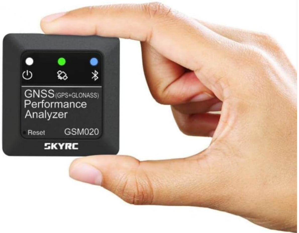
Figure 2: Compact size of the GNSS Performance Analyzer (40x40x17mm, 38g).
