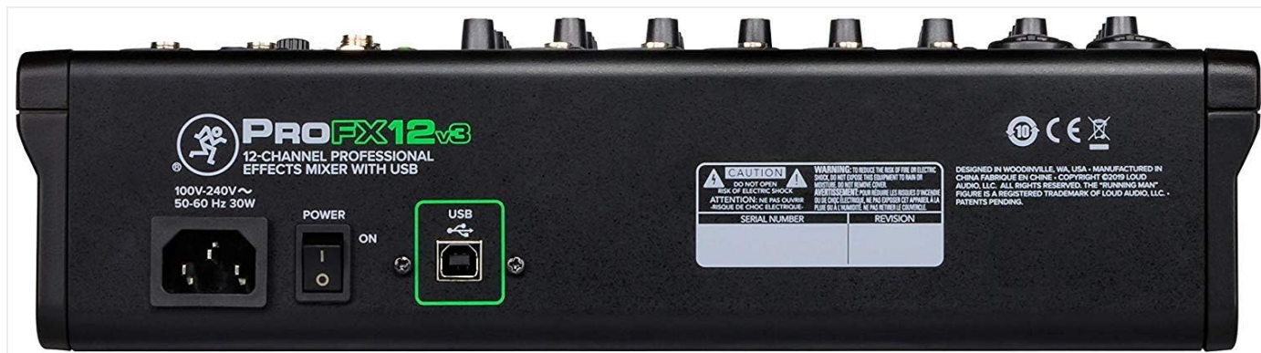
Figure 1: Rear panel connections of the Mackie ProFX12v3 mixer. This view highlights the power input, USB port for computer connectivity, and main audio outputs including XLR and 1/4-inch jacks.
