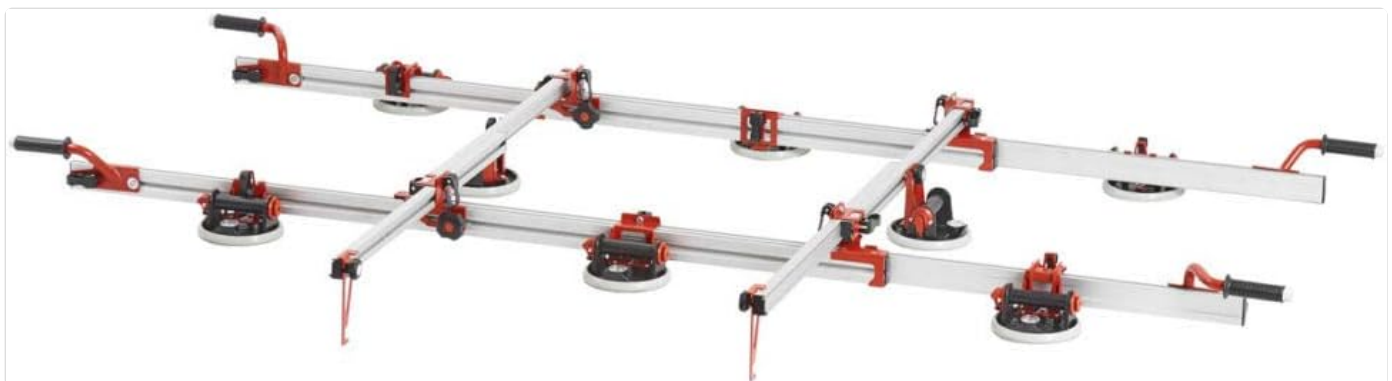
Figure 1: The Raimondi Easy-Move RV175 tile transport system, fully assembled and ready for use. It shows the two main aluminum profiles, crossbars, eight vacuum suction cups, and ergonomic handles.
