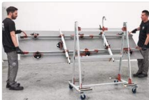
Figure 7: The Raimondi Easy-Move RV175 system actively transporting a large tile, demonstrating its use in conjunction with a tile support stand for efficient handling.
