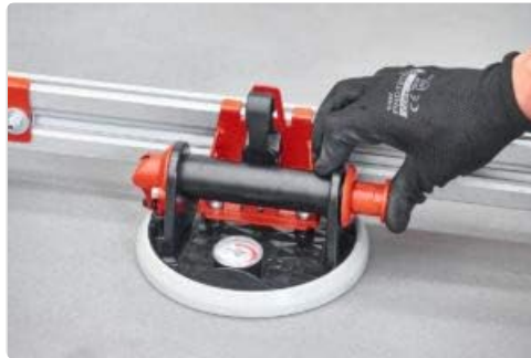
Figure 5: A hand operating the vacuum pump on a suction cup. The red line indicator on the pump cylinder is visible, indicating the need to pump until it disappears for full vacuum.
