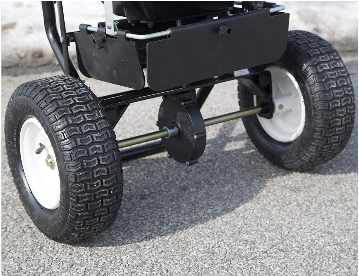
Figure 5.2: Close-up view of the wheels and the gear-driven spreading mechanism, which activates as the spreader is pushed.
