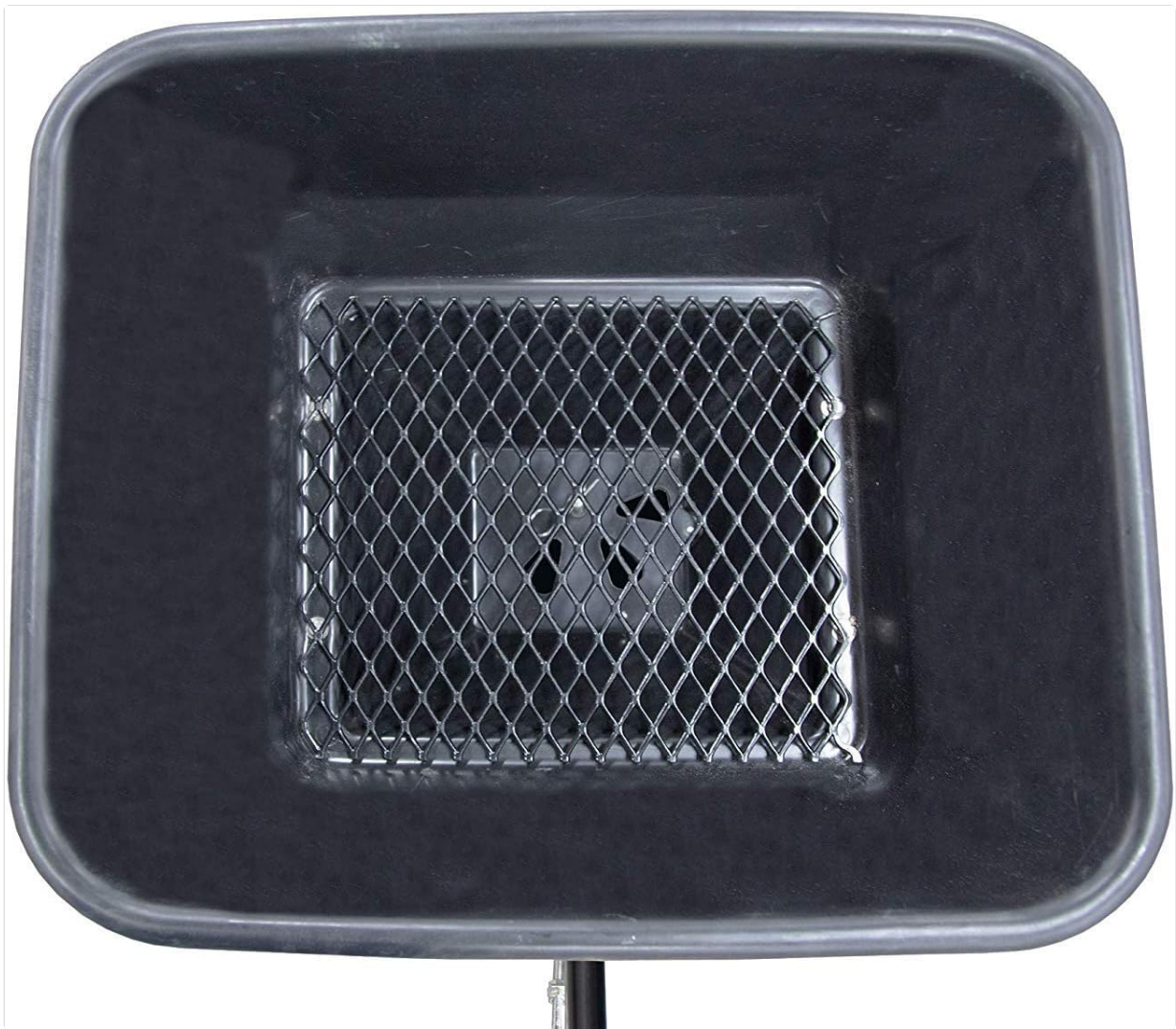
Figure 5.1: Top view of the hopper, showing the protective grate to prevent large clumps from entering the spreading mechanism.
