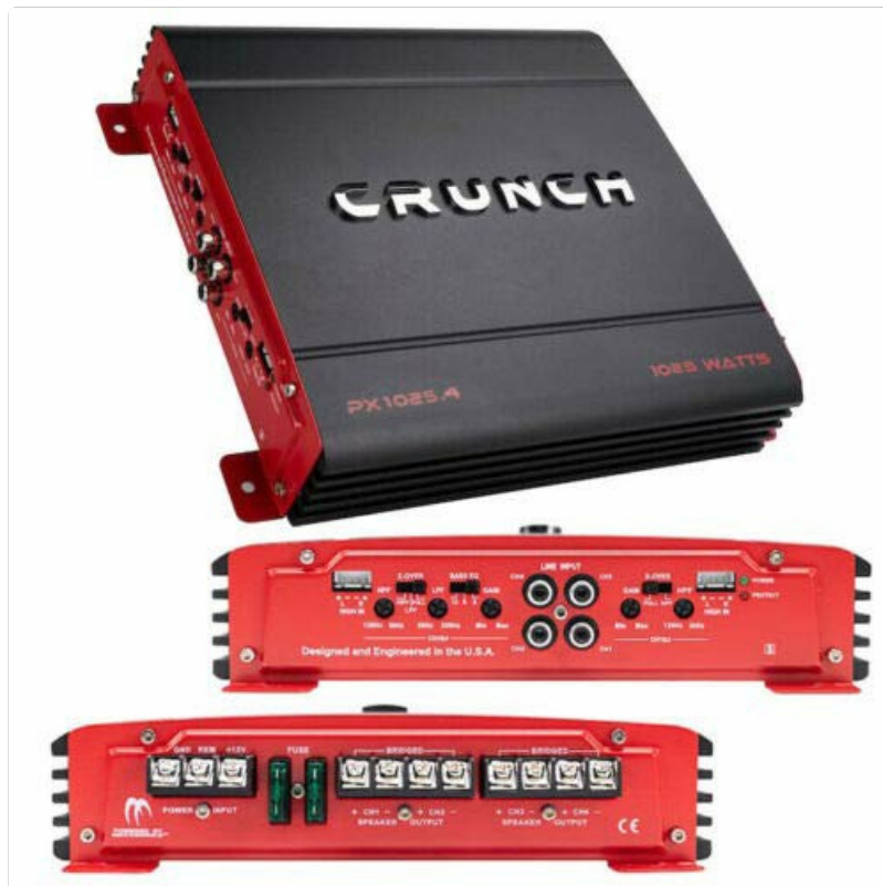
Image: This image displays both the input and output sides of the Crunch PX-1025.4 amplifier. The top view shows the RCA inputs, gain controls, and crossover settings. The bottom view shows the power, ground, remote, and speaker output terminals, along with the fuse block.
