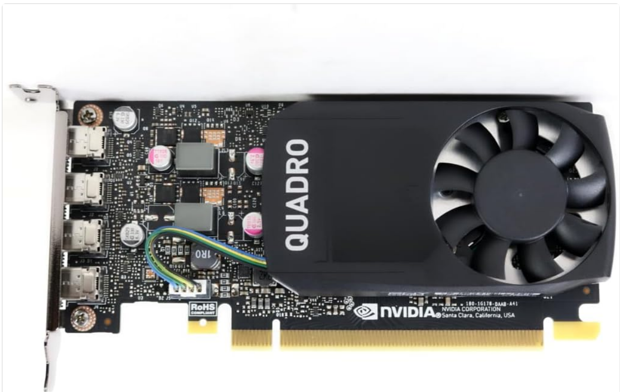
Figure 2.2: Top-down view of the PNY Quadro P620 graphics card, showing the fan and heatsink assembly.
