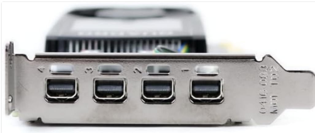
Figure 3.1: Close-up view of the four Mini DisplayPort outputs on the PNY Quadro P620 graphics card.
