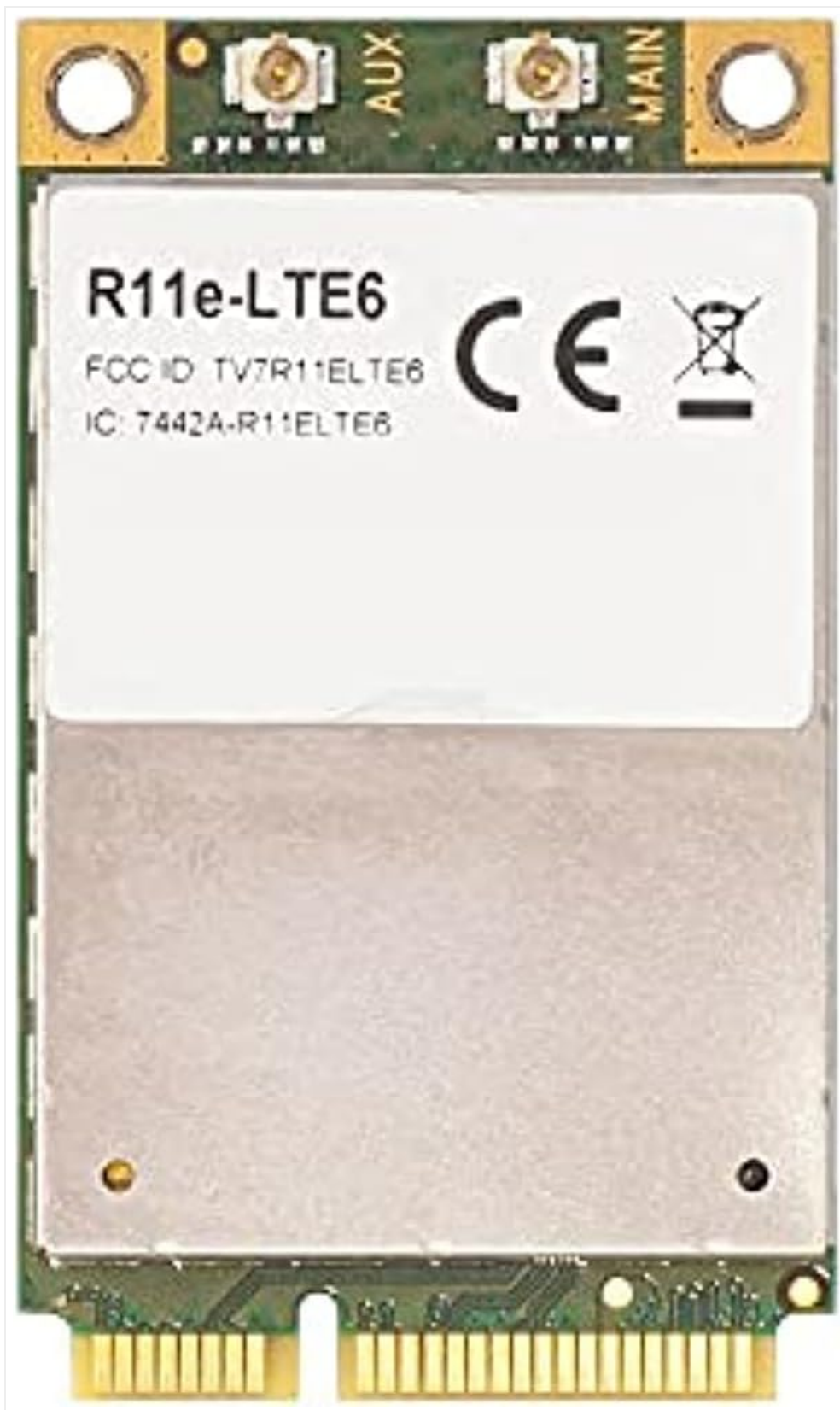
Image 1: Front view of the MikroTik R11e-LTE6 miniPCI-e Card. This image displays the top side of the card, highlighting the R11e-LTE6 model designation, regulatory markings (FCC ID, CE), and the two gold-plated antenna connectors labeled 'MAIN' and 'AUX' at the top edge. The miniPCIe connector pins are visible at the bottom.
