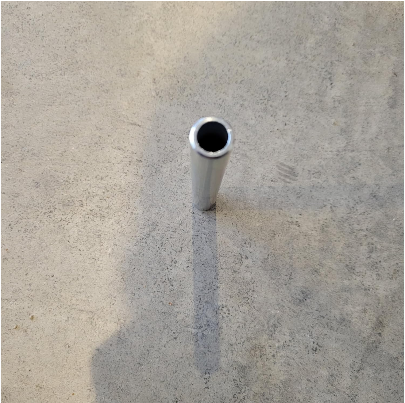
Figure 3.3: Close-up of the mounting post. This image shows the hollow nature of the cylindrical mounting post, which is inserted into the miter saw's clamp slot.
