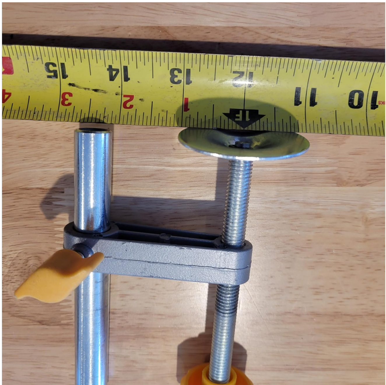
Figure 8.1: Clamp dimensions. This image shows the clamp alongside a measuring tape, indicating its approximate size and the length of the threaded screw.
