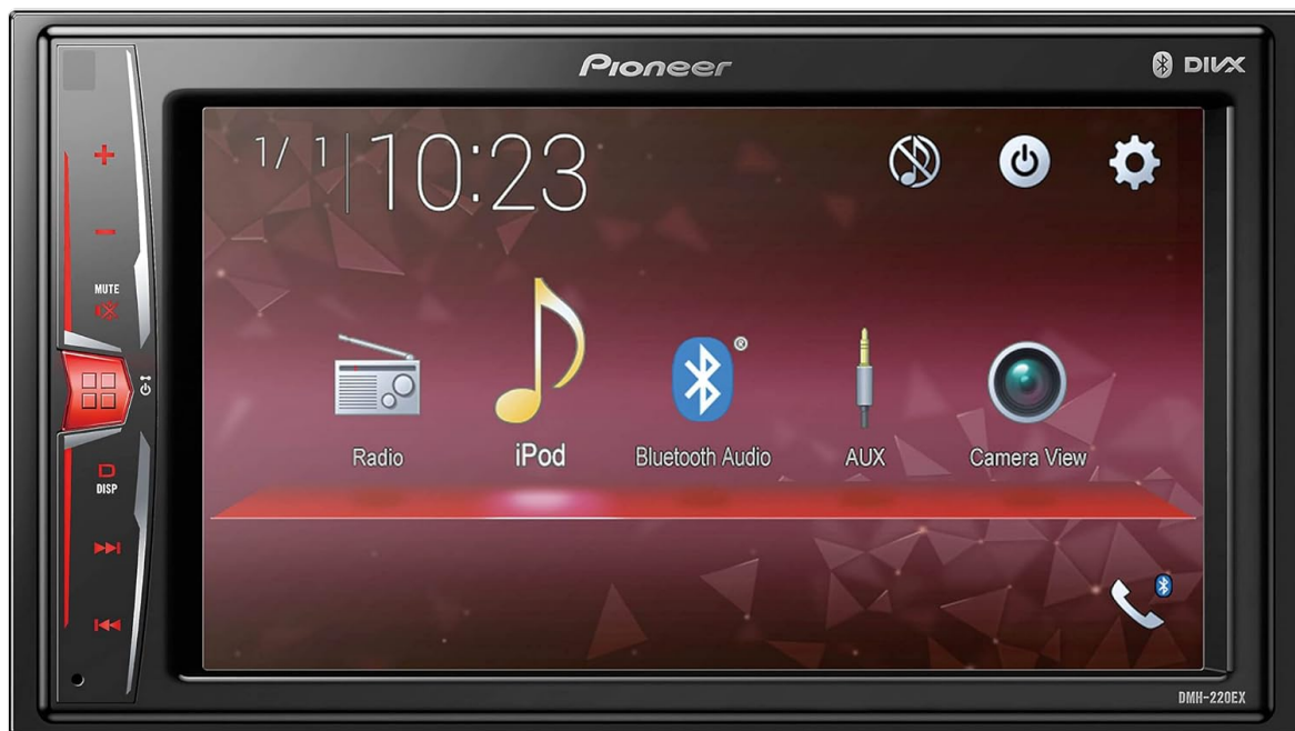
Figure 3: Main menu screen of the Pioneer DMH-220EX, showing options for Radio, iPod, Bluetooth Audio, AUX, and Camera View.
