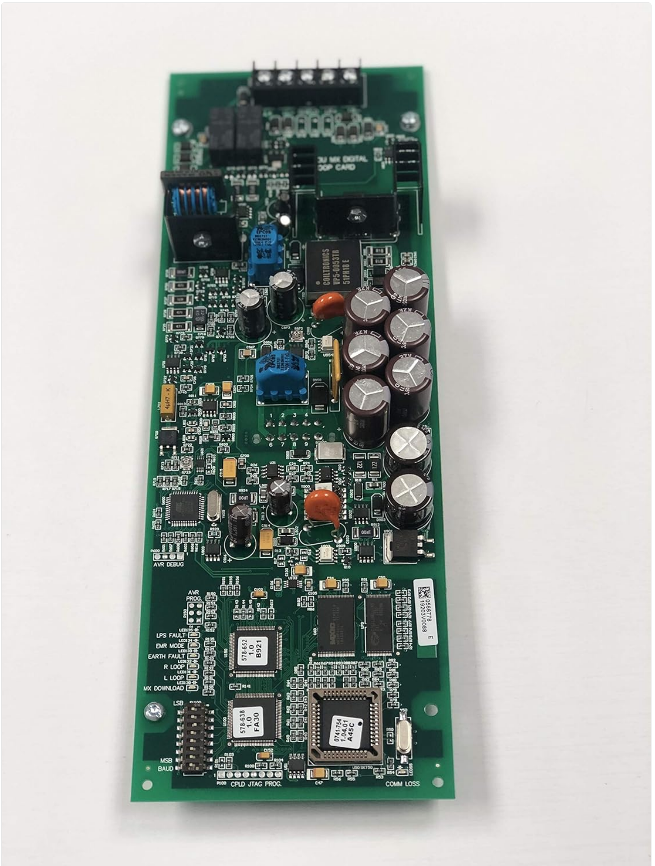
Image: A close-up view of the SIMPLEX 4100-6077 MX Loop Module, showing its green circuit board with various electronic components, including integrated circuits, capacitors, and resistors. The module is depicted in a vertical orientation, ready for installation into a control panel chassis.
