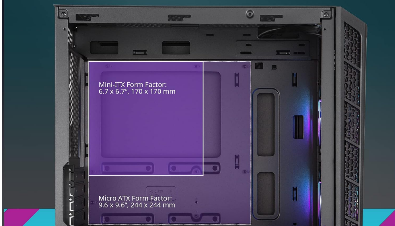
Image: Interior of the case highlighting the motherboard mounting area, compatible with Mini-ITX and Micro-ATX form factors.
