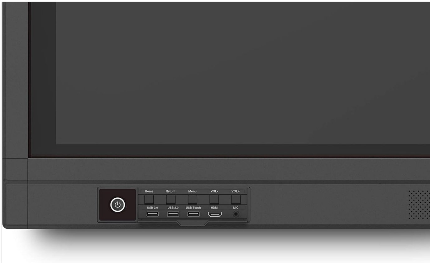
Figure 3: Detail of the control panel and connectivity ports located at the bottom of the display.
