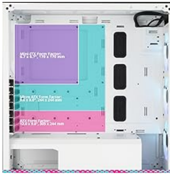
Figure 2.1: Diagram illustrating supported motherboard form factors and their placement within the case.
