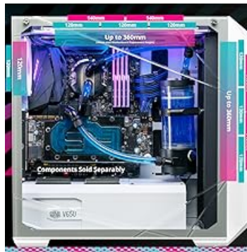
Figure 2.3: Overview of fan and radiator mounting locations and supported sizes.
