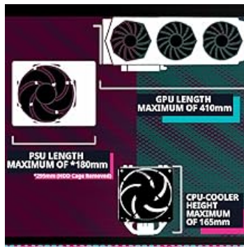
Figure 2.2: Diagram showing maximum clearances for GPU, PSU, and CPU cooler.
