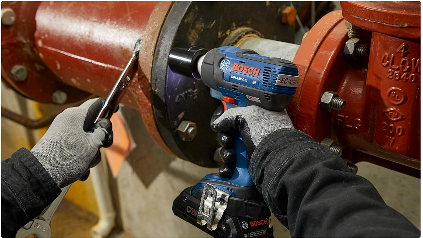
Figure 5.2: The impact wrench in use on a pipe flange, illustrating its utility in plumbing and industrial maintenance tasks.
