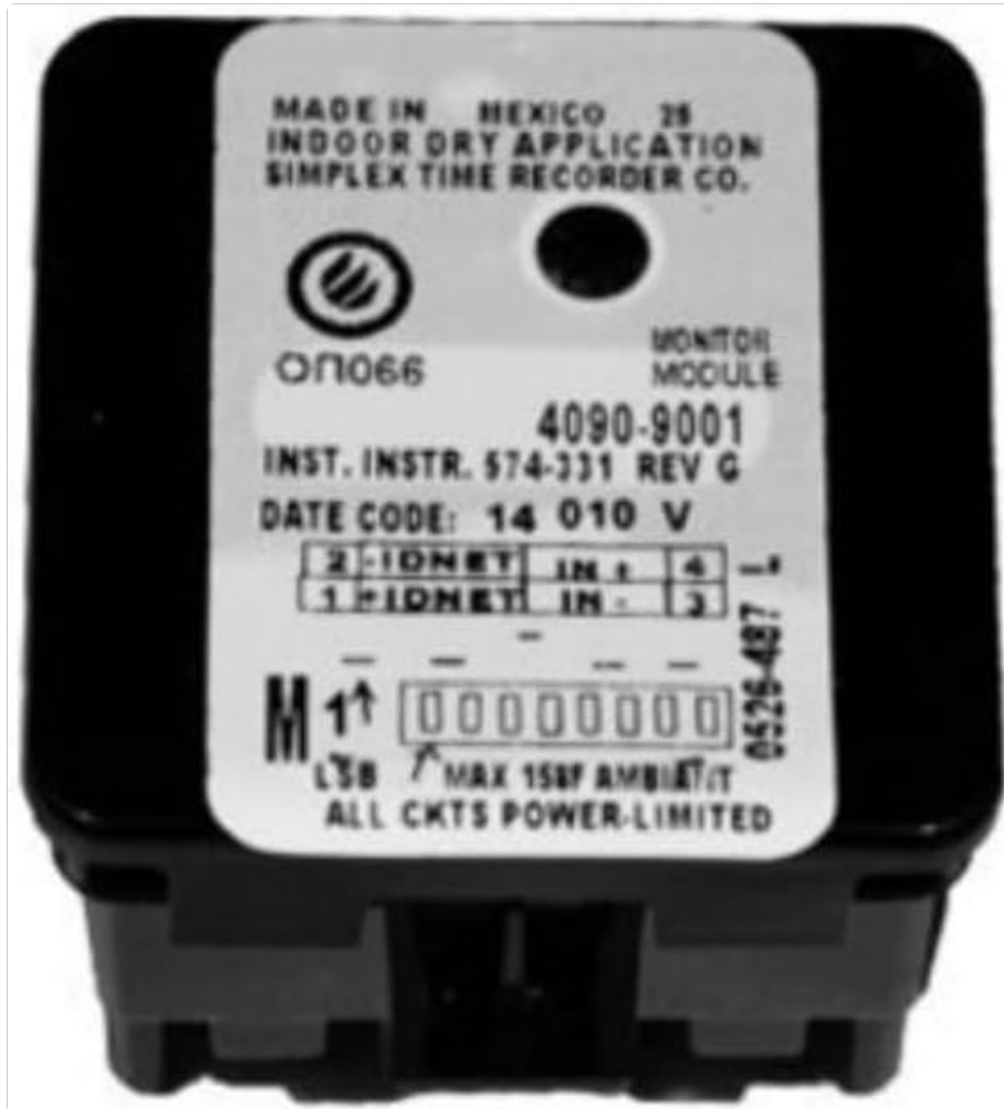
Figure 3.1: Front view of the Simplex 4090-9001 module, clearly showing the IDNET input/output terminals (1-4) and the module's model number and revision information.
