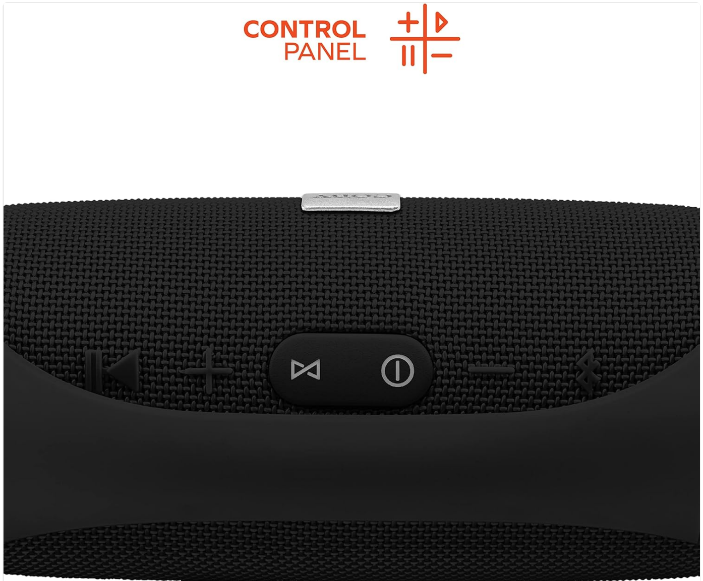
Image: A close-up view of the speaker's top control panel, showing buttons for power, play/pause, volume up/next track, and volume down/previous track.
